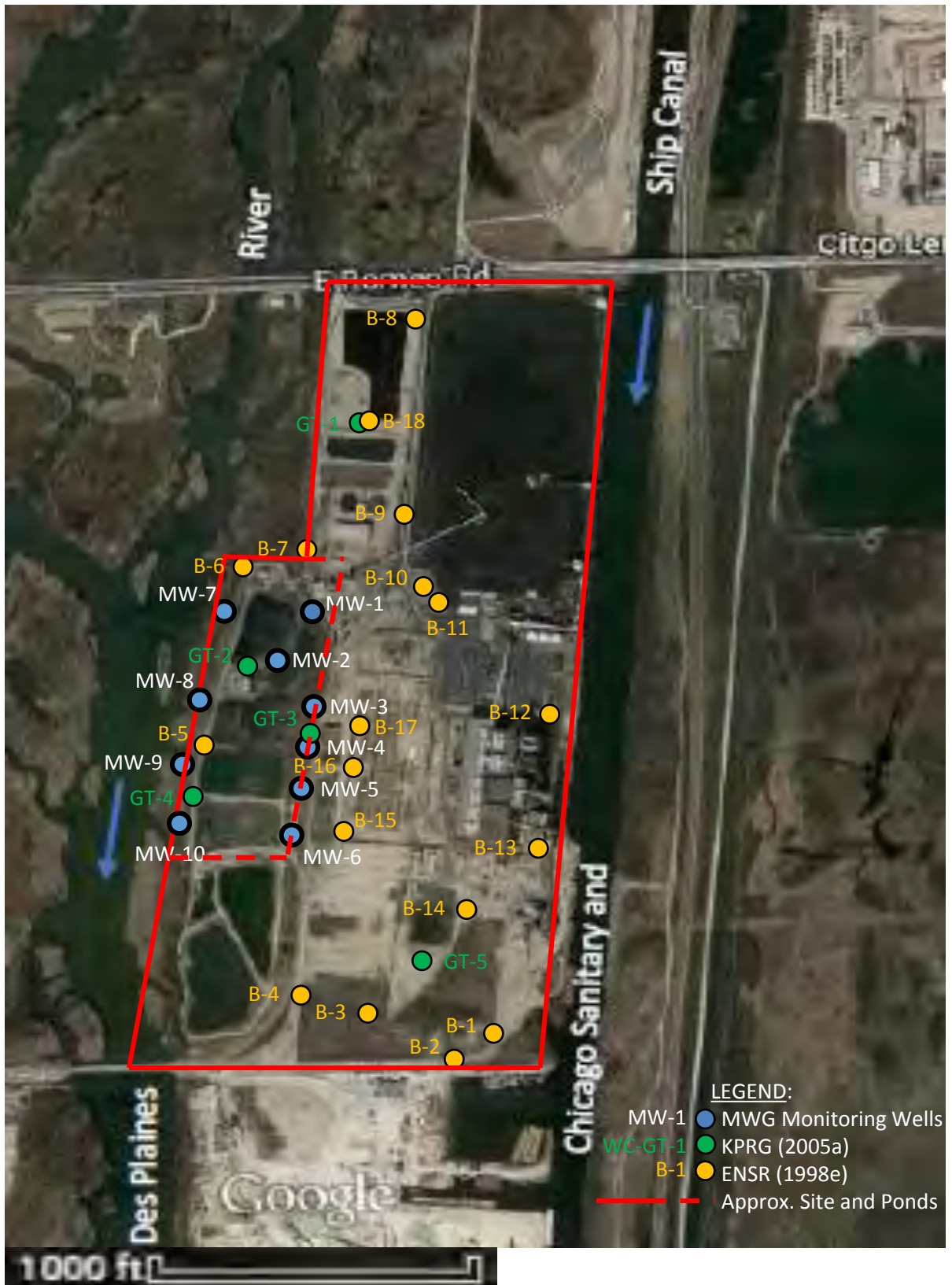
Figure 4 Will County Soil Boring Locations (PCB 2013-015)
